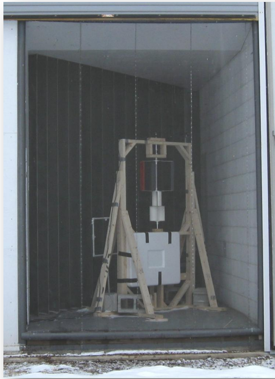
Figure 10. Turbine model in contraction room of wind tunnel during wind tunnel testing.
