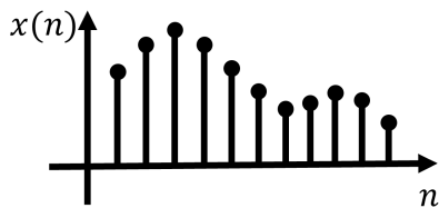
FIG. 1: A digital signal with sample number, n , on the horizontal axis.
