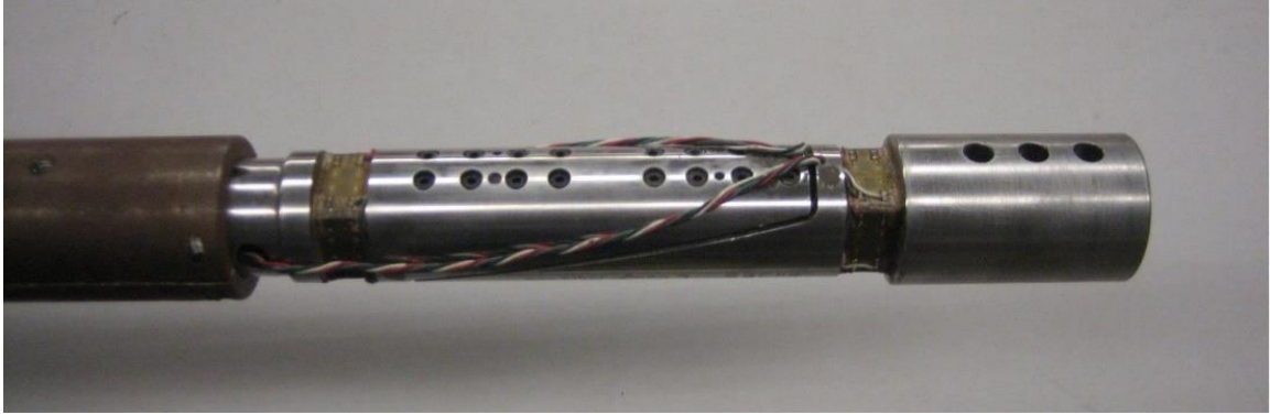
Figure 29. Six component internal force balance [6]
