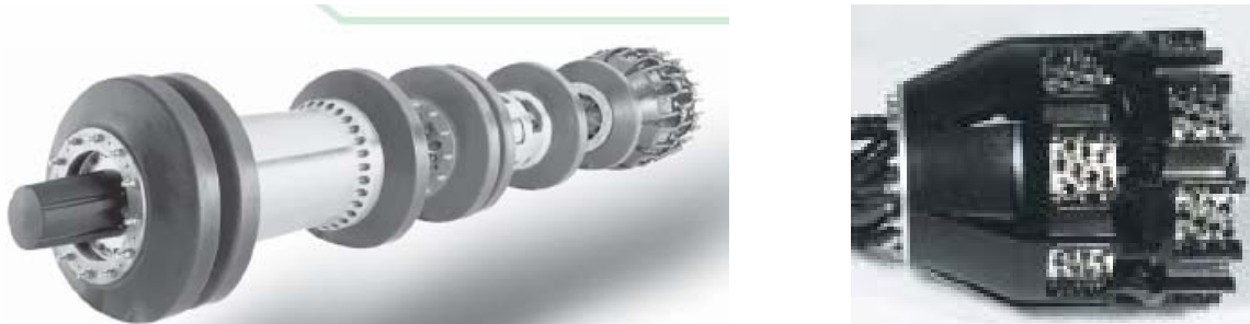
Figure 2-6: Ultrasonic ILI with a Close-Up of the Instrumentation.
