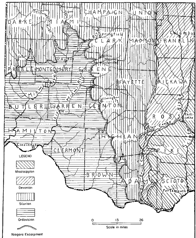
FIGURE 15. Geologic map of southwestern Ohio showing the distribution of the rock systems, the course of the Niagara Escarpment, and the drainage.
