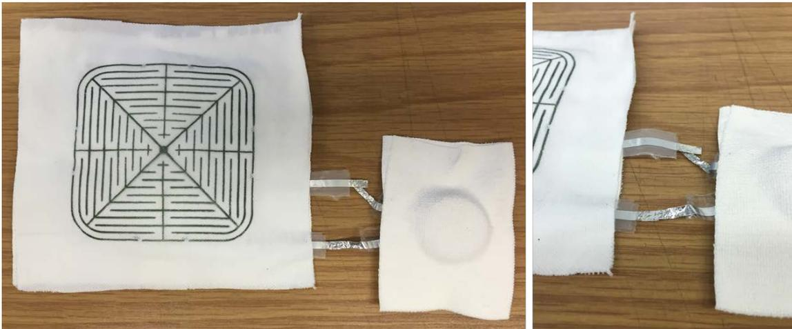
Figure 3: Inherited bandage including 6V battery pack. Bandage is comprised of a polyester fabric facing the wound, conductive circuit, cotton padding to absorb wound exudate, and an adhesive backing to seal the dressing. Notice the bandage and battery pack are connected by joining aluminum tape leads.
