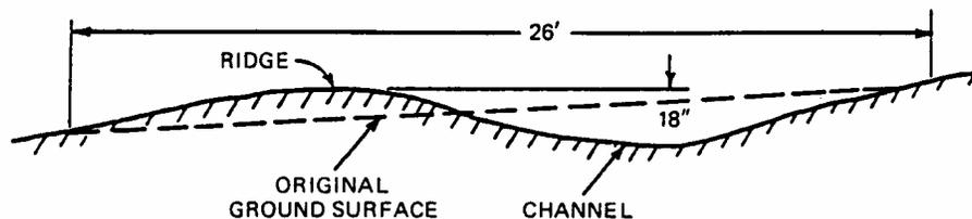
Figure 2-6 Cross section of a typical diversion.
