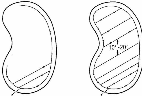
Figure 4-3 Recommended drain line placement in a California green; (A) under conditions of low rainfall or a steeply sloped green; (B) under conditions of high rainfall or a gently sloped green.
