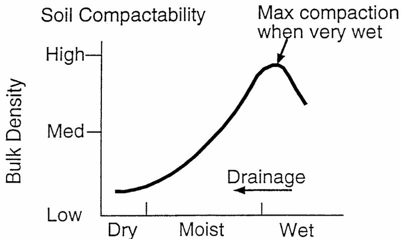
Figure 1-5 Relation between soil compaction and soil moisture for a cohesive soil.
