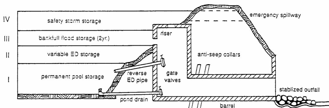
Figure 5-5 Cross section of a deeper, stormwater wetland micropool.
