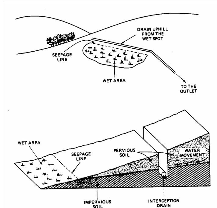
Figure 3-5 A subsurface interceptor used to drain a hillside seep.
