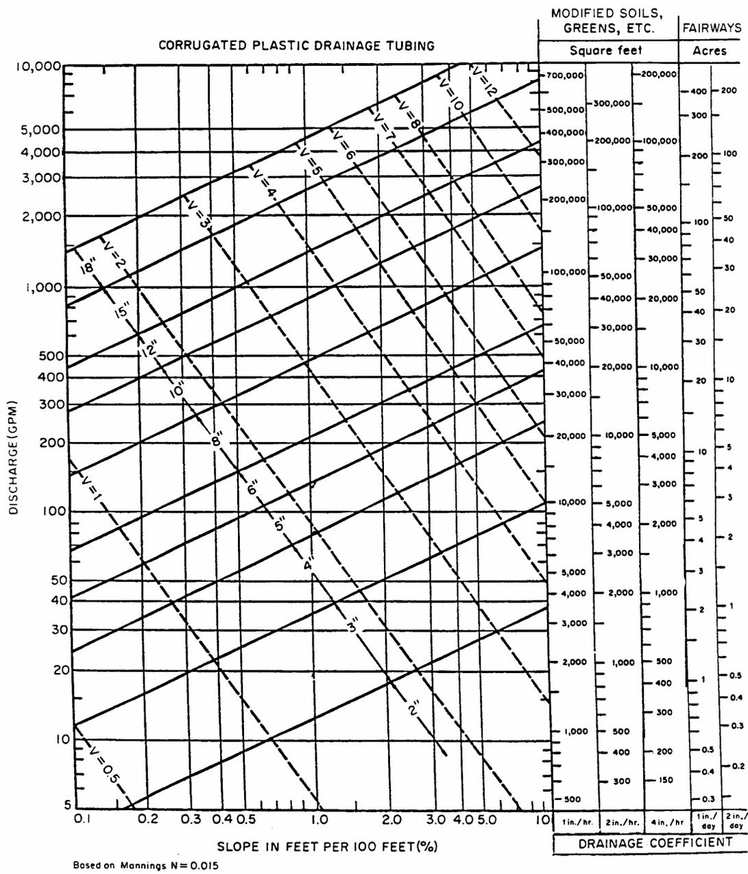
Figure 3-3 Drainage capacity chart for corrugated plastic drainage tubing.
