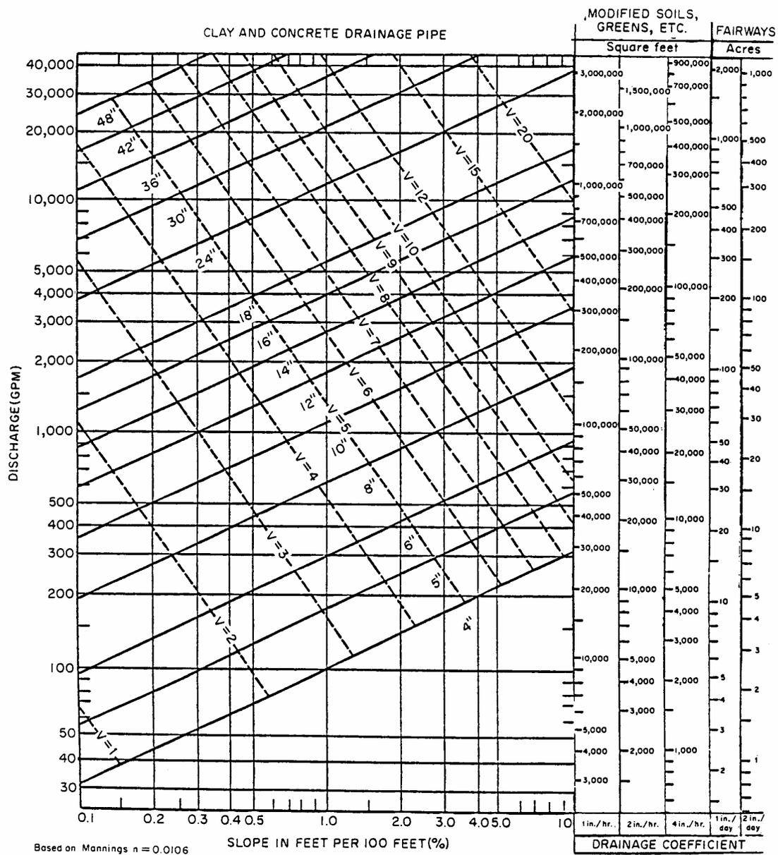
Figure 3-2 Drainage capacity chart for smooth-walled plastic, clay and concrete drainage pipe.
