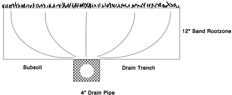
Figure 4-5 Pathways of water movement to the drain line trench of a California green.
