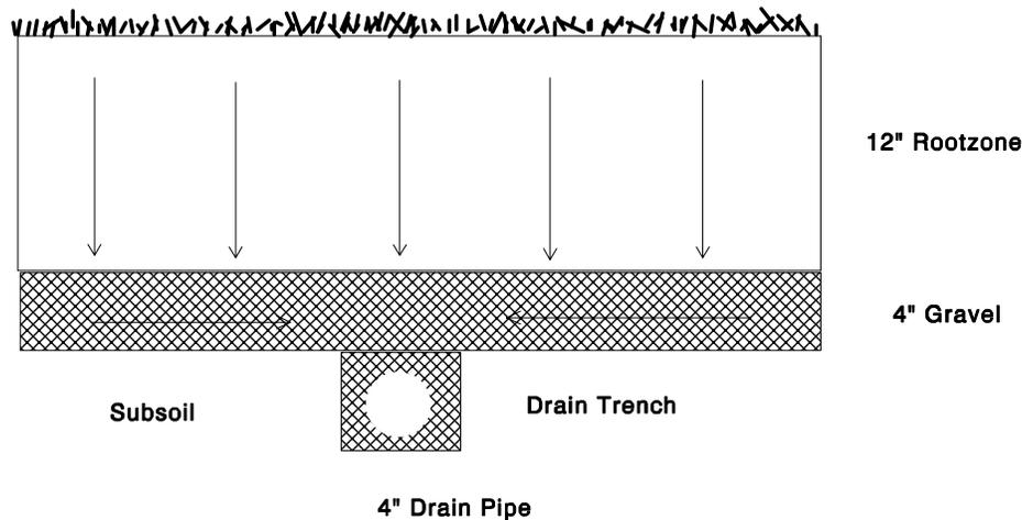
Figure 4-6 Pathways of water movement to the drain line trench of a USGA green.
