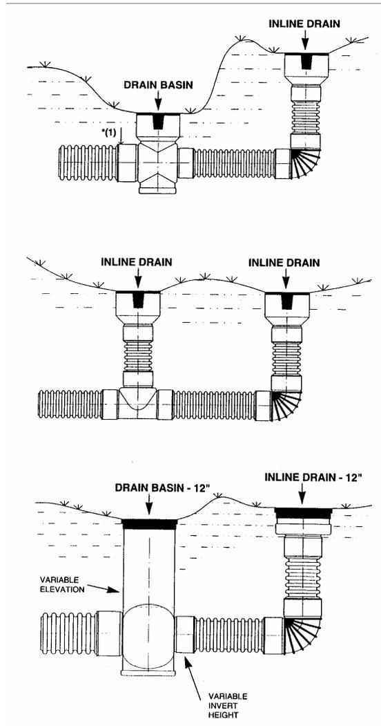
Figure 2-7 Typical surface inlet installations.
