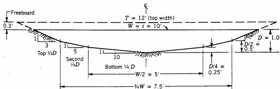
Figure 2-4 Cross section of a parabolic shaped channel.
