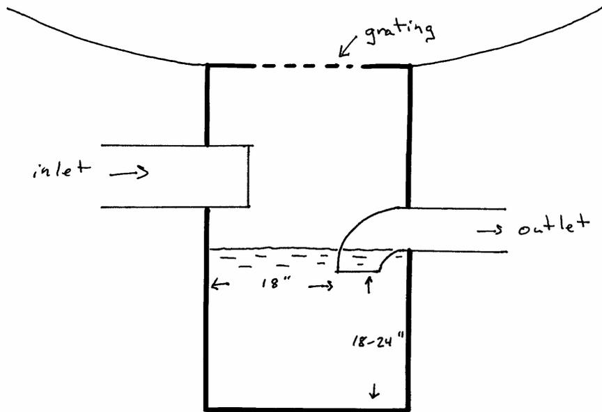
The key to properly designing this flow control structure is through use of the orifice equation. This equation is given as:
