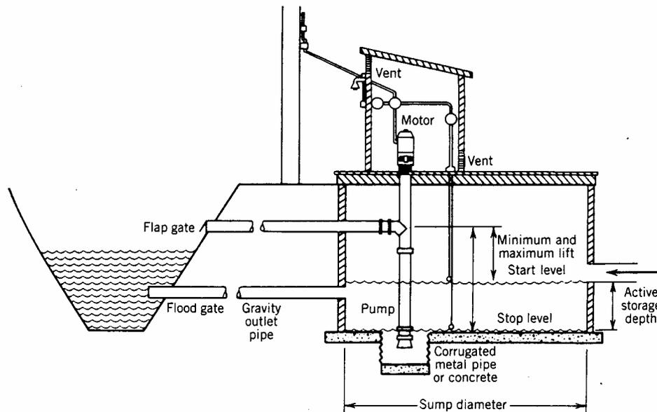
Figure 5-3 A pumped outlet.
