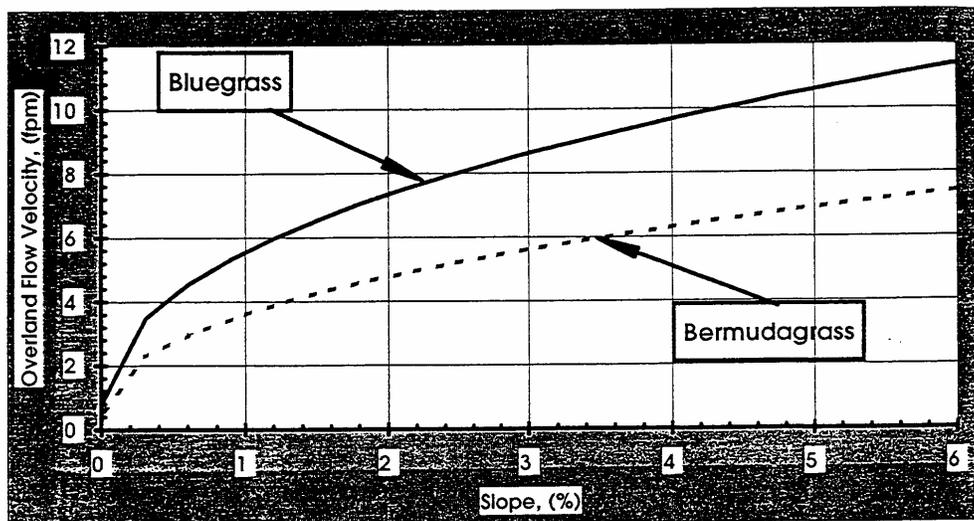
Figure 1-1 Overland flow velocities through turf canopies.
