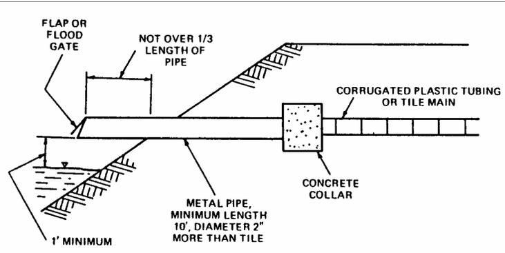
Figure 5-1 A classical drainage system outlet.
