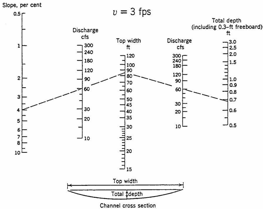
Figure 2-5 Design nomograph for a grass-lined channel with flow velocities limited to 3 feet per second.
