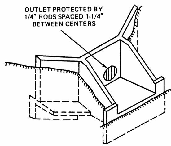
Figure 5-2 A concrete headwall for a classical outlet.
