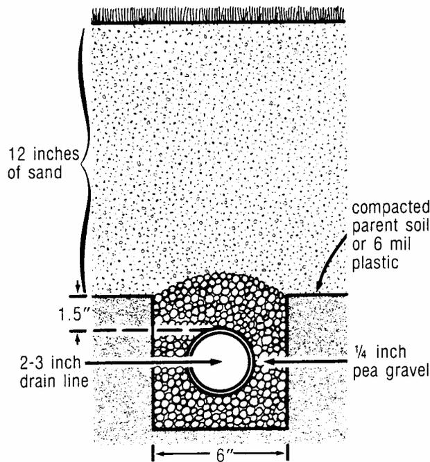
Figure 4-2 Soil profile of a California system green.
