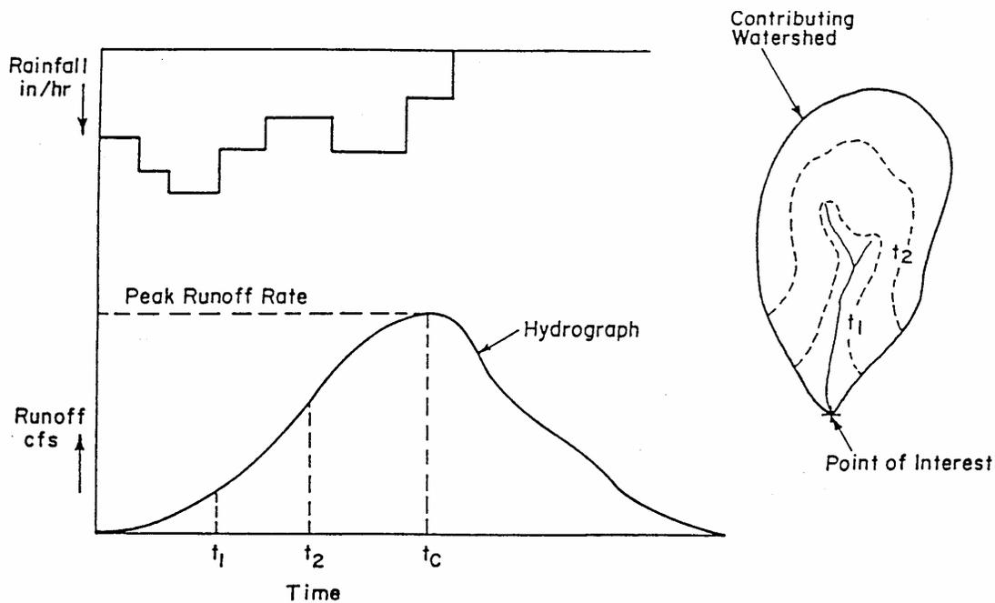
Figure 1-4 A conceptual model of watershed hydrologic processes.
