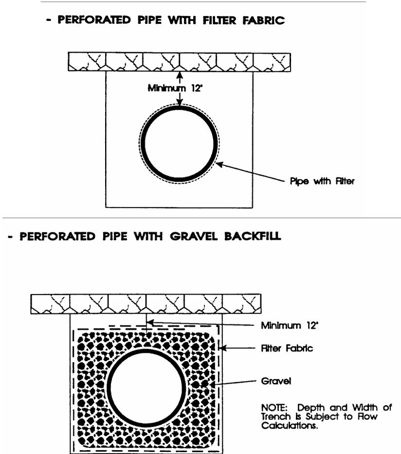
Figure 5-4 The two possible configurations for a subsurface reservoir.
