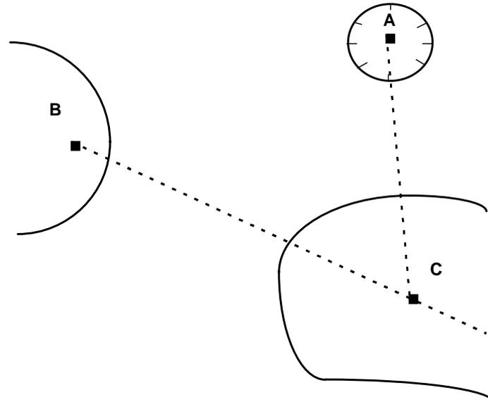
Figure 2-8 Example of pipe sizing for multiple surface inlets.
