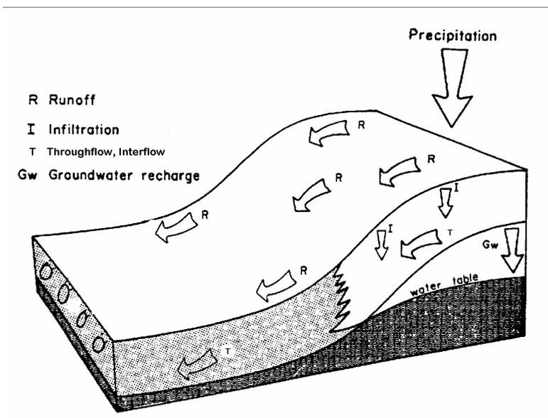
Figure 1-2 Flow paths for water movement on hillslopes.
