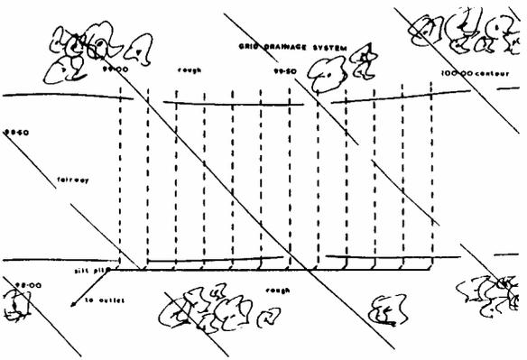
On fairways a grid system of drains can be used where the fall is diagonally across the line of play.
