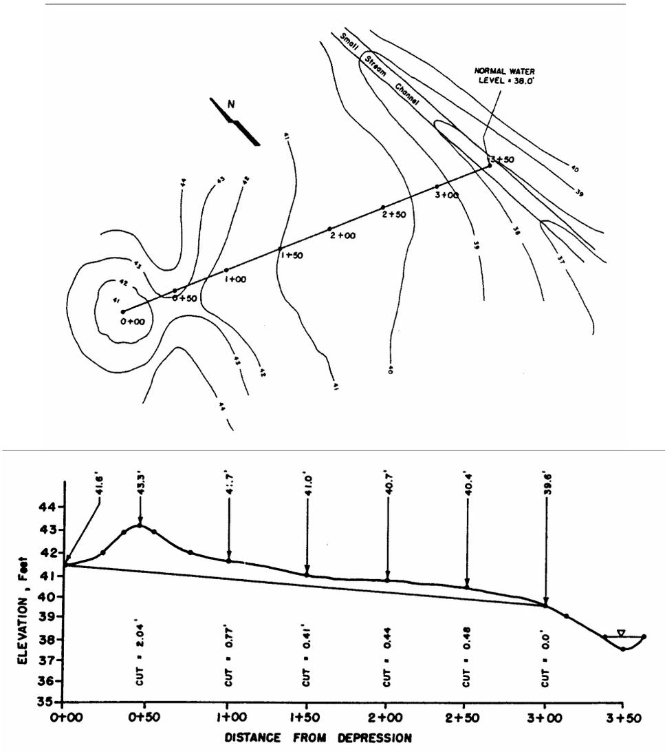
Figure 2-3 An example of surface drainage for a depression.
