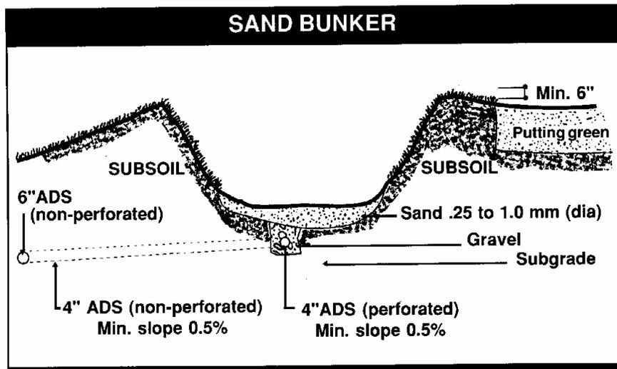
Figure 4-4 Cross sectional view of a generalized sand bunker.
