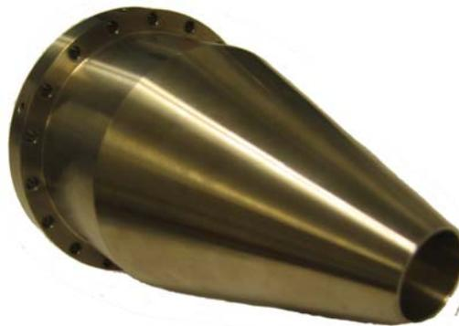
**Figure 3.1 – Picture of the Mach 0.9 converging nozzle used to obtain all the data shown in this thesis. The nozzle is made of stainless steel and has an exit diameter of 1 inch.**
