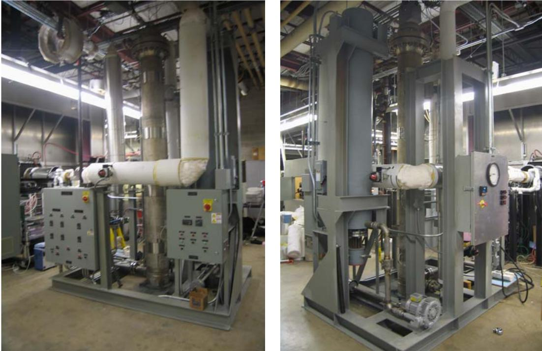
**Figure 3.5 – (Left) The storage heater used to provide heat to the jet facility. (Right) The other side of the storage heater showing the jet facility control panel from Figure 3.3 (the heater is undergoing modification in both of the pictures here).**
