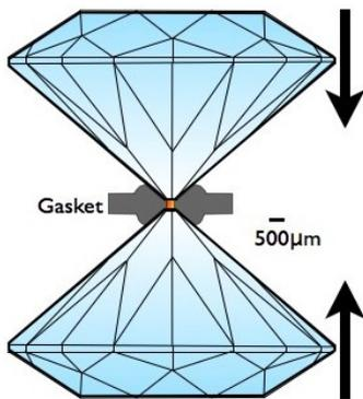
Figure 2. Diamond and sample set-up within the LHDAC.
