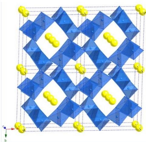
Figure 3. Tunneling of the hollandite structure in the direction of the  $c$ -axis through edge-sharing (Si, Al)O<sub>8</sub> octahedra. (Si, Al)O<sub>8</sub> octahedra are represented by the blue polyhedra, while the site for +1 charge cations is represented with yellow balls. The smaller blue balls represent either Si or Al.
