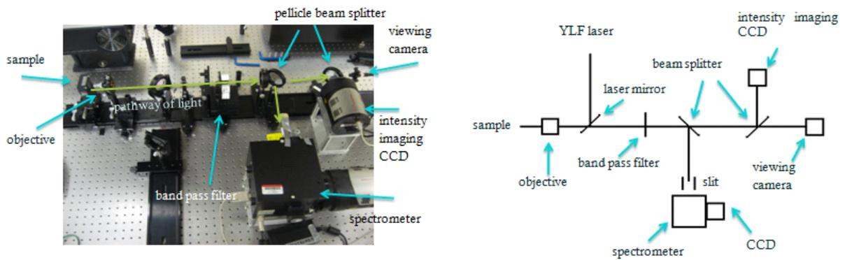
Figure 11. Laser-heating optics table in the high-pressure mineral physics lab at Ohio State University (left) and schematics of optics table (right)
