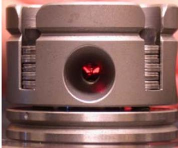
Figure 1. Laser-heated diamond anvil cell (LHDAC), which measures about 3 inches in diameter and 2 inches tall.
