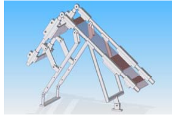
Figure 3: Design solid model. The base at the lower left of the mechanism is stationary while the slider at the lower right of the mechanism is able to translate back and forth.
