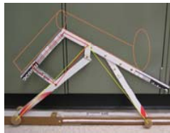
Figure 4: Cardboard prototype of design. Mechanism is a combination of a slider-rocker and 4-bar linkage.
