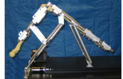
Figure 6: Final assembled device. Sawbones of the femur, tibia, and fibula represent the approximate location of the cadaver specimen.
