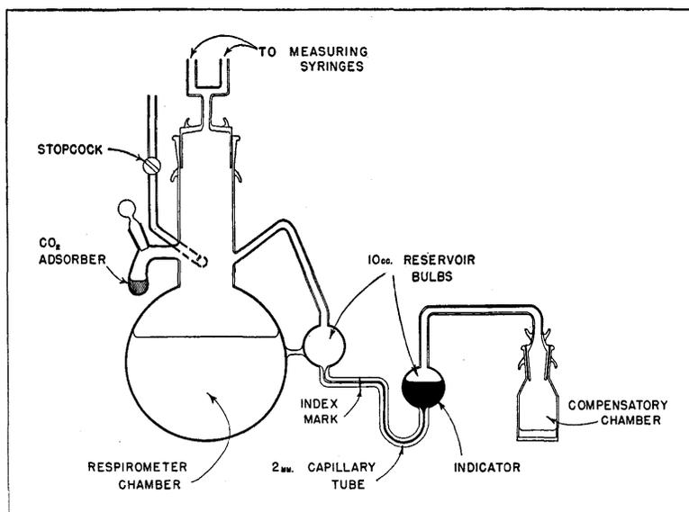
FIGURE 1. The volumeter used for respirometric studies (see text for discussion).
