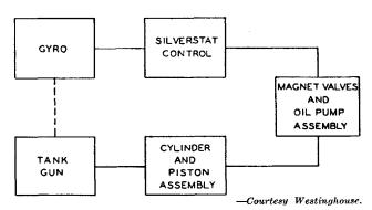
(above)—Block diagram of stabilizer—The gyro control is mounted on the gun breech. Tank fluctuations over rough terrain cause the gyro to precess, contacting silverstat leaves and changing current flow to magnet valves. The position of the valves in seats is determined by current energizing the magnet coils. As one valve moves away from the seat, the other moves farther into its seat.
