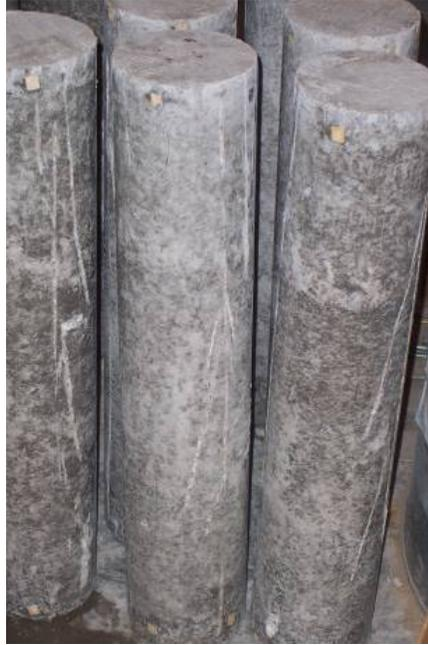
Figure 3.1 – Base Columns Before Retrofitting (Miller 2006).
