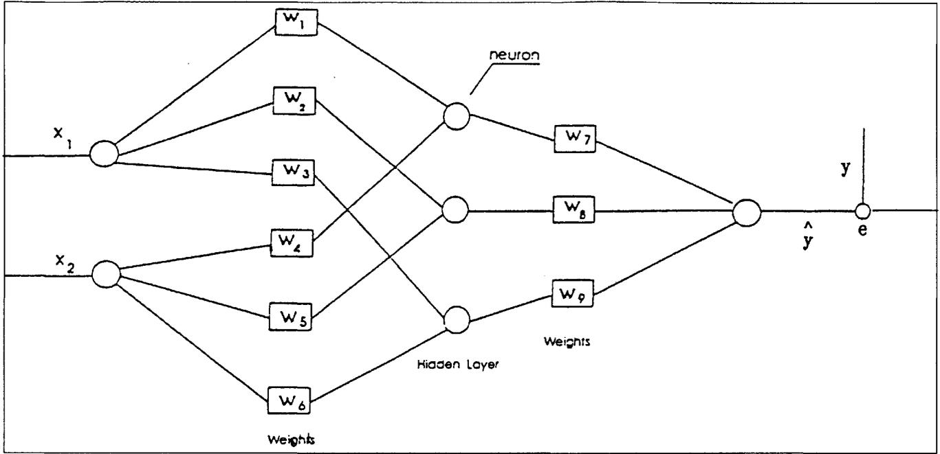
FIGURE 1. A neural network model with three layers and nine weights.
